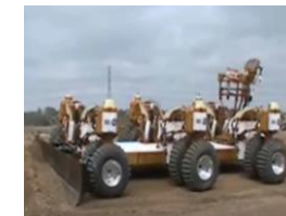
RASSOR, LANCE, and LSMS work together to pile regolith on top of shelter and form berms
