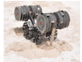
RASSOR, LANCE, and LSMS work together to pile regolith on top of shelter and form berms
